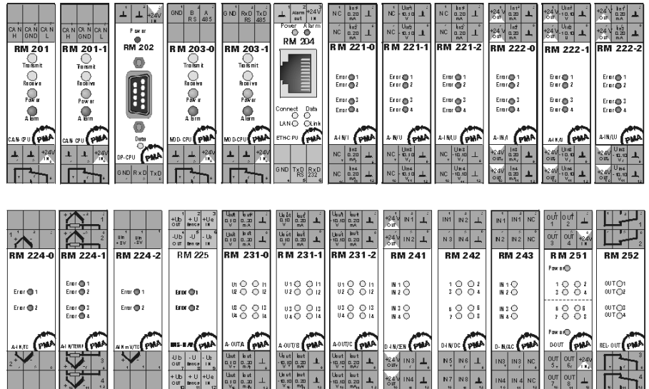
Fig.4 : Display Elements and Connections of RM 200 modules
